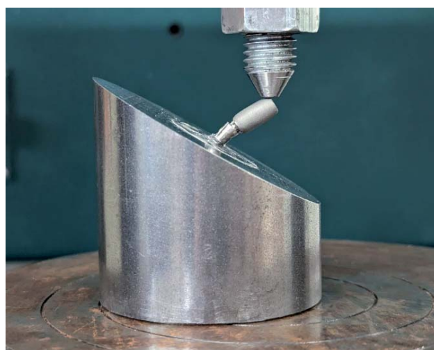
Fig. 3. Compression testing with a visible implant deformation
