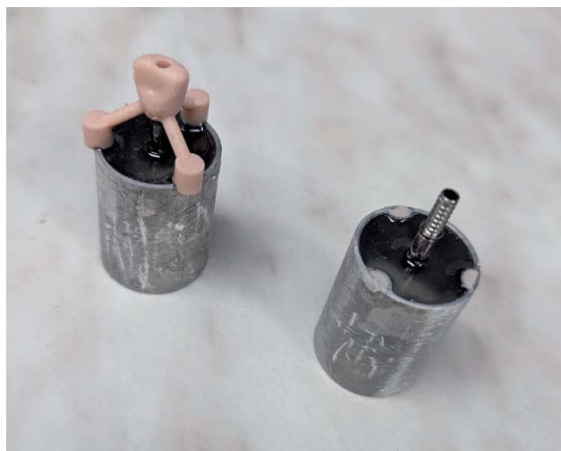
Fig. 2. On the left implant with a 3D printed guide, on the right implant with a detached guide
