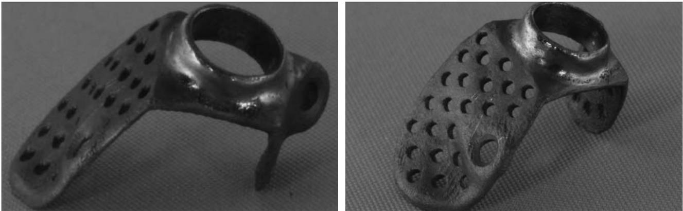
**Fig. 6.** 3D printed device used to protect Trefoil prosthesis implant stability, created using Titanium powder (DMLM technology)
