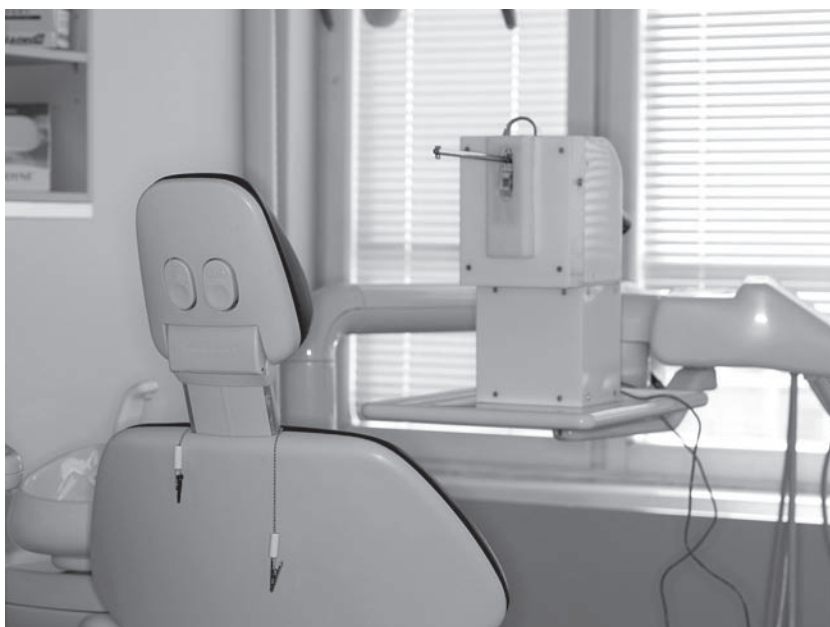
Fig. 2. Pressure sensitive instrument modified to test passive tactile threshold in the dental chair
