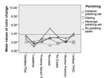
**Fig. 4.** Graphical representation of mean ( $\Delta E$ ) colour changes after repolishing procedures of provisional materials soaked in mix of sunset yellow and quinoline yellow 3% solution for all polishing groups
