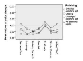
**Fig. 3.** Graphical representation of mean ( $\Delta E$ ) colour changes after repolishing procedures of provisional materials soaked in distilled water (control) for all polishing groups
