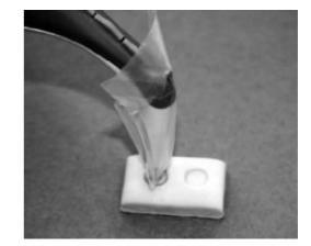
Fig. 2. Spectrophotometer tip placed against a specimen in a custom silicone holder
