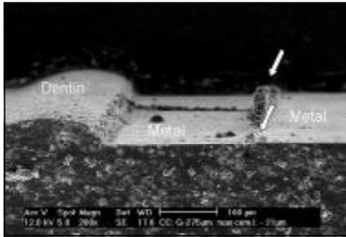
**Picture 14.** Cement adaptation to metal (measurement point A). Negative image of the test surface illustrating the defect of cement at the metal/cement interface.
