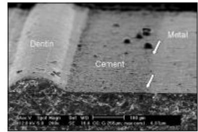
**Picture 13.** Cement adaptation to metal (measurement point A). Negative image of the test surface illustrating a smooth and uninterrupted transition from the cement to the metal.
