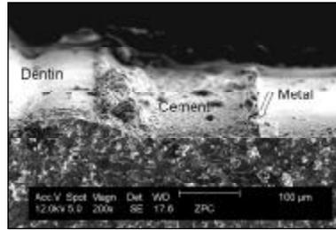
**Picture 15.** Cement adaptation to metal. Negative image of the test surface illustrating the defect of cement at the metal/cement interface (measurement point A).
